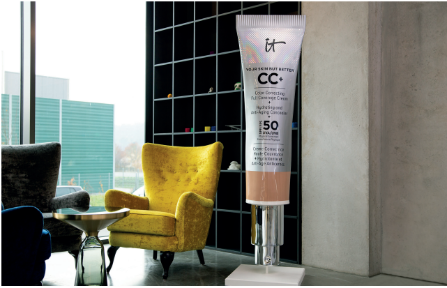
Fig. 3. Accomplished advertising sculpture for L'Oréal with GDP corpus, generated by photopolymerization of a highly-viscous gel © FIT AG/Lisa Kirk
