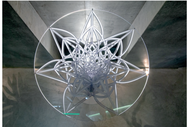
Fig. 10. The ornamental lattice geometry of this table was created by using stereolithography © FIT AG/Lisa Kirk
