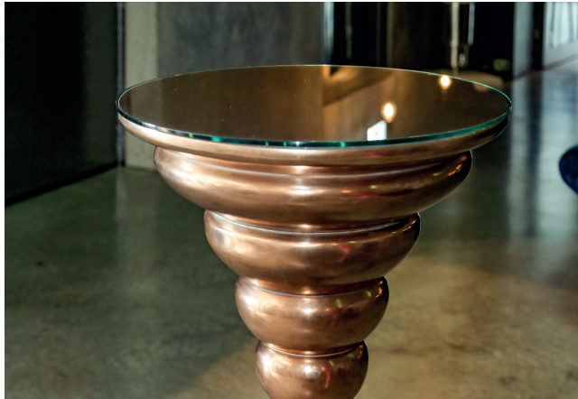
Fig. 11. The entire object was printed via GDP as a hollow article, filled with foam and coated with bronze
